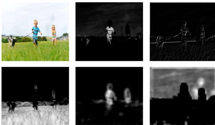
Fig. 3. Input image and sample activation maps from a typical CNN. (Top row) Input image and two activation maps from earlier layers showing part objects like t-shirts and features like contours. (Bottom row) Activation maps from later layers with more meaningful activations like fields, people, and sky, respectively.
